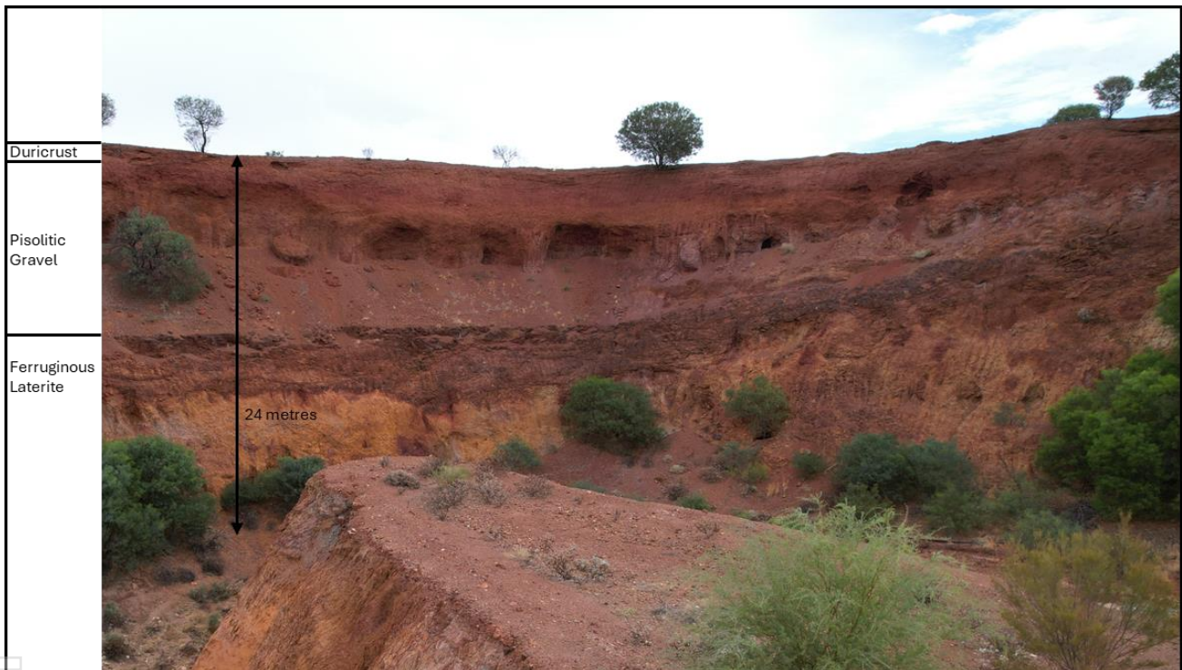
Figure 1 - Looking south toward the Cable Pit south wall illustrating an indicative regolith profile within the starter pit.
