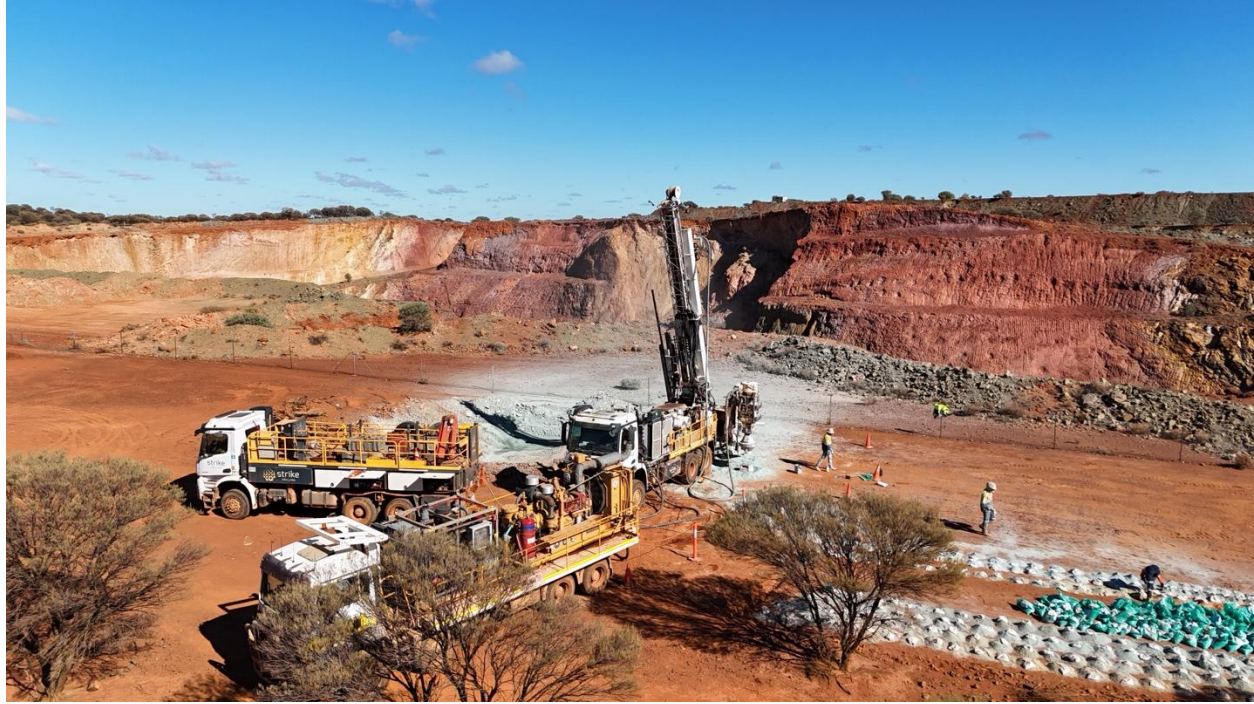
Figure 1 – RC drill rig operating at Mt Fisher. May 2026
