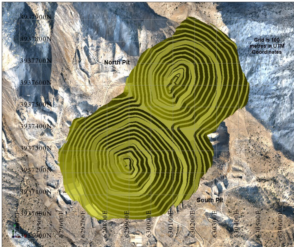
Figure 40 Final Open Pit Design
