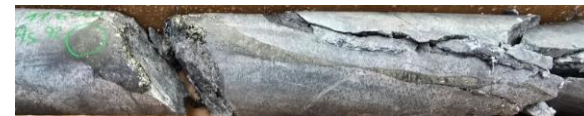
Chalcopyrite sulphide within a c-type vein within altered porphyry from 400m in 25LLDD0070
