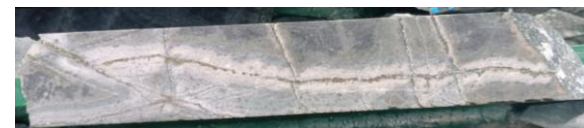
Pyrite–Chalcopyrite sulphide veining with albite selvedge's from 1,434m downhole in 25LHDD071
