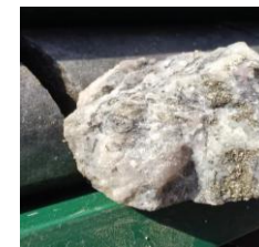
Pyrite–Chalcopyrite sulphide quartz vein from 1,389m downhole in 25LHDD071
