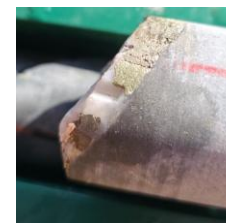
Pyrite–Chalcopyrite–Molybdenite sulphide veining from 1,351m downhole in 25LHDD071
