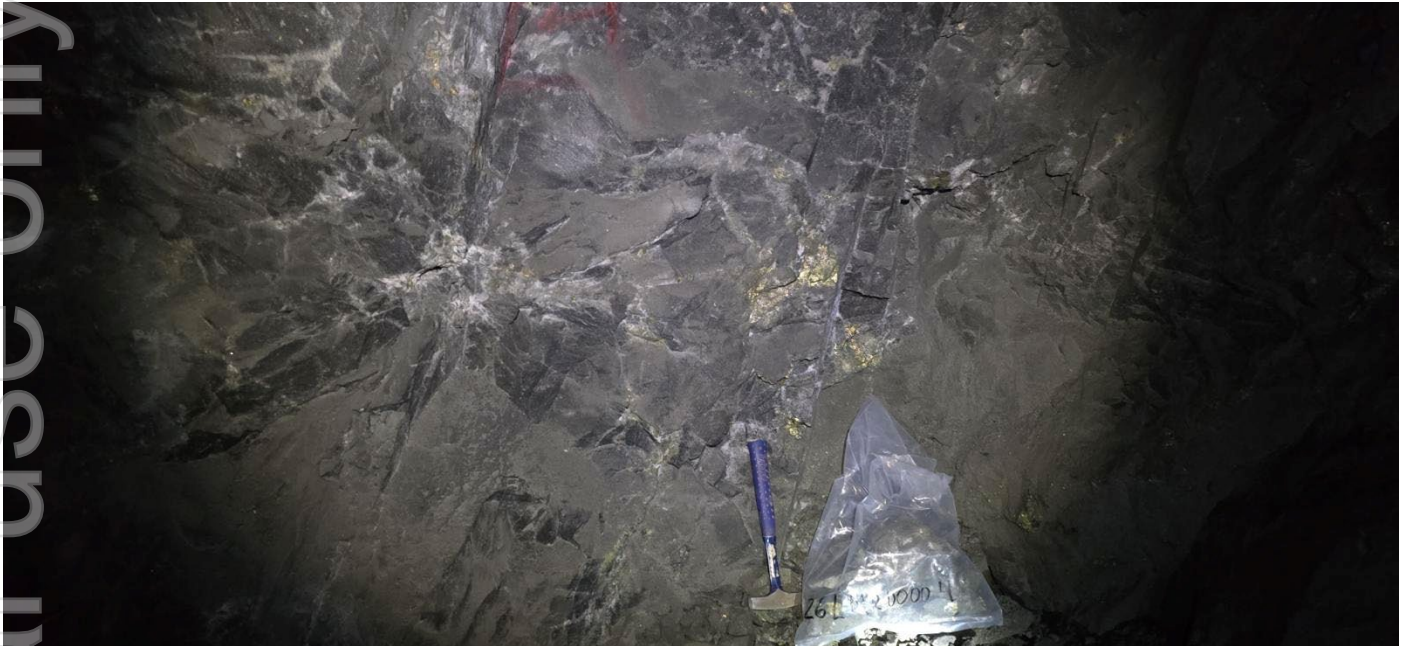
Photo 5. Underground rock chip sample 26MLR00004 from the Los Morados Prospect, showing copper sulphide associated with structurally controlled quartz-sulphide veining (see Table 1).
