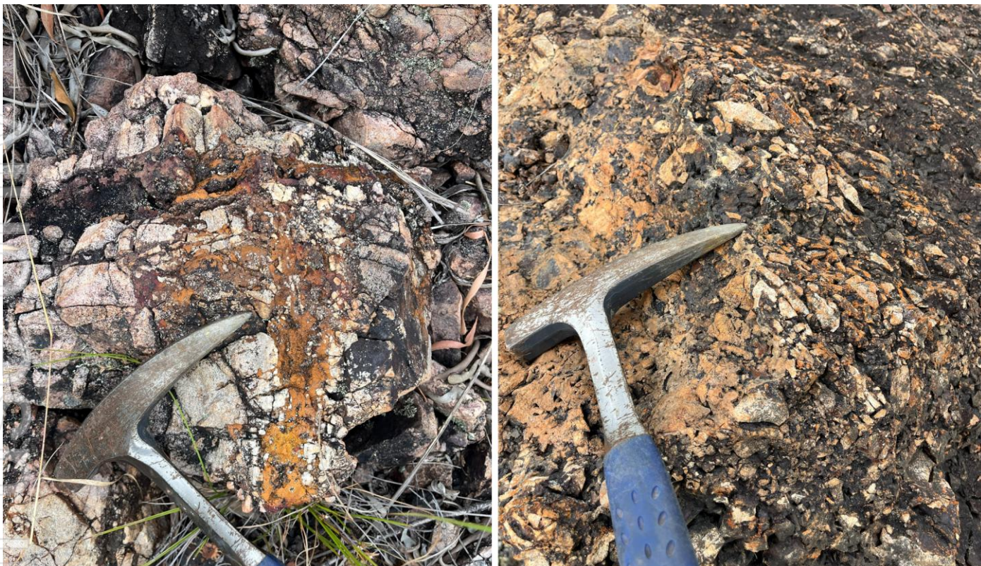
Figure 6 left: Mt Gossan sandstone breccia. Right: clast supported brecciated sandstone with iron oxide after sulphide matrix infill.
