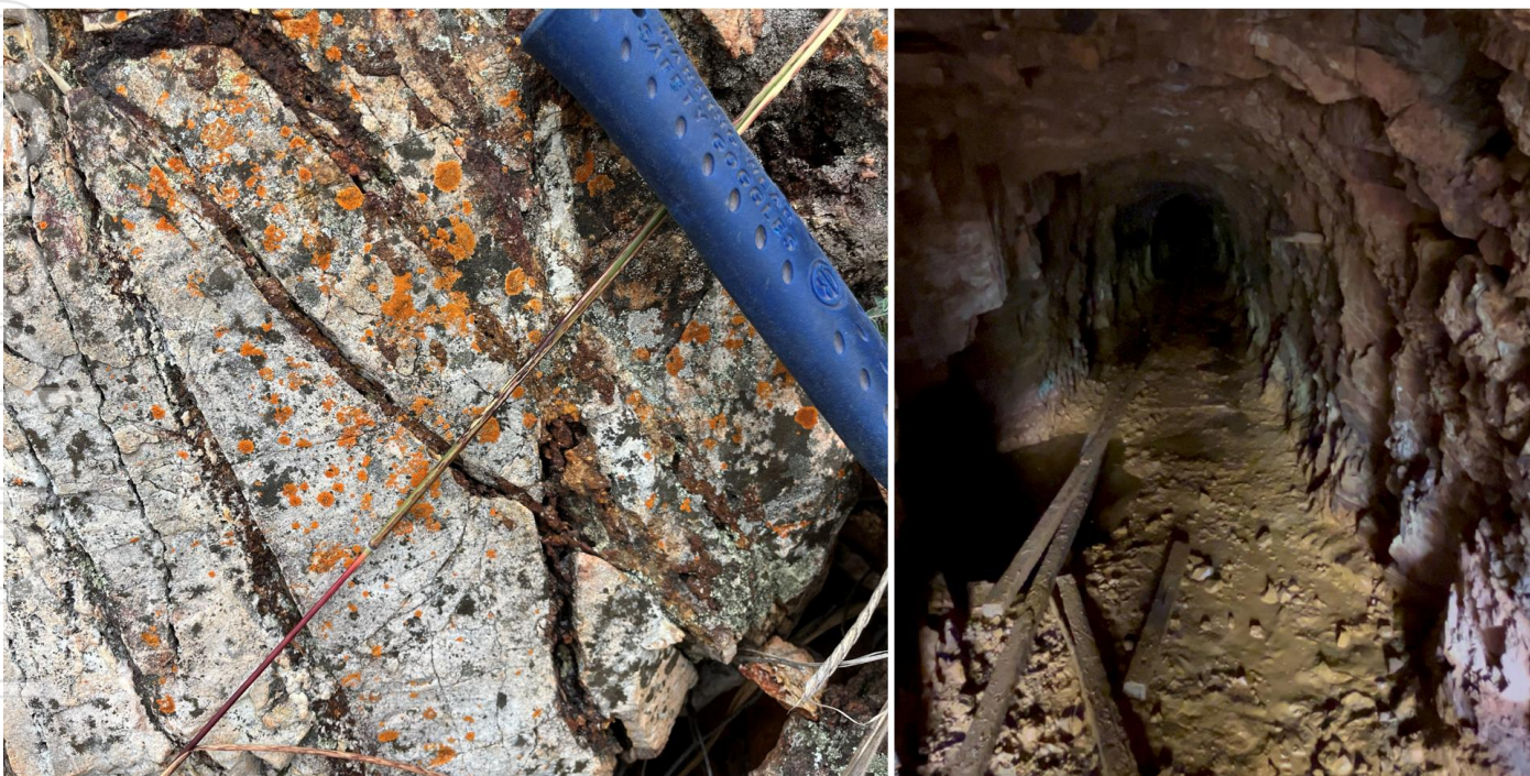
Figure 7 Left: Sandstone cut by sheeted quartz + iron oxide after sulphide veins and stockwork veins containing iron oxide after sulphide. Right: Mt Gossan mine adit.
