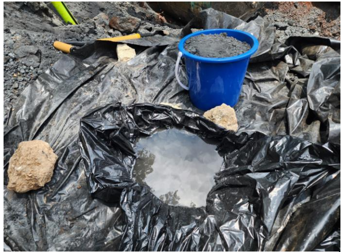
Figure 6. Field in-situ bulk density test at Ira Miri using the Excavation and Water-Fill Method. Excavated material was weighed, and void volume was determined by filling the plastic-lined excavation with a measured volume of water.
