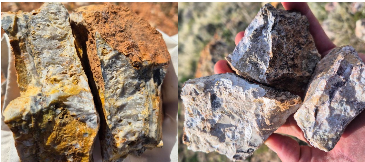
Figure 4: Photographs (left) bladed textured silica vein IBLH03 (1.66 g/t Au, 65.9 g/t Ag) and (right) silica-altered porphyritic rock with lithic fragments IBLH06 (1.46 g/t Au, 53.8 g/t Ag).
