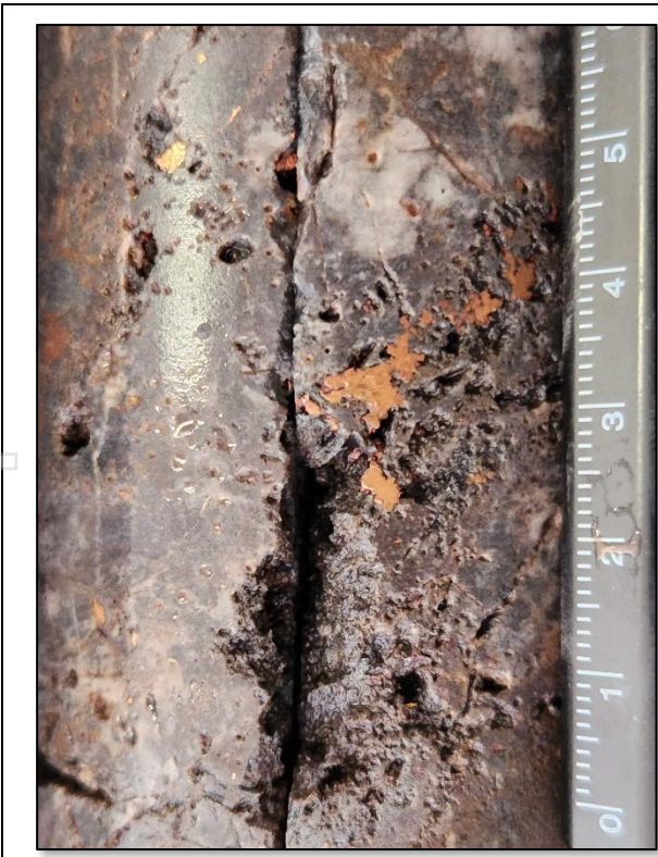
IMAGE 5 a and b: Hematite, quartz, jasper, copper sulphide, copper breccia (BBDD0050 @195m).
