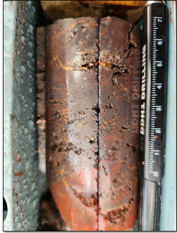
IMAGE 4 a and b: Hematite, quartz, jasper, copper sulphide, copper breccia (BBDD0050 @194m).
