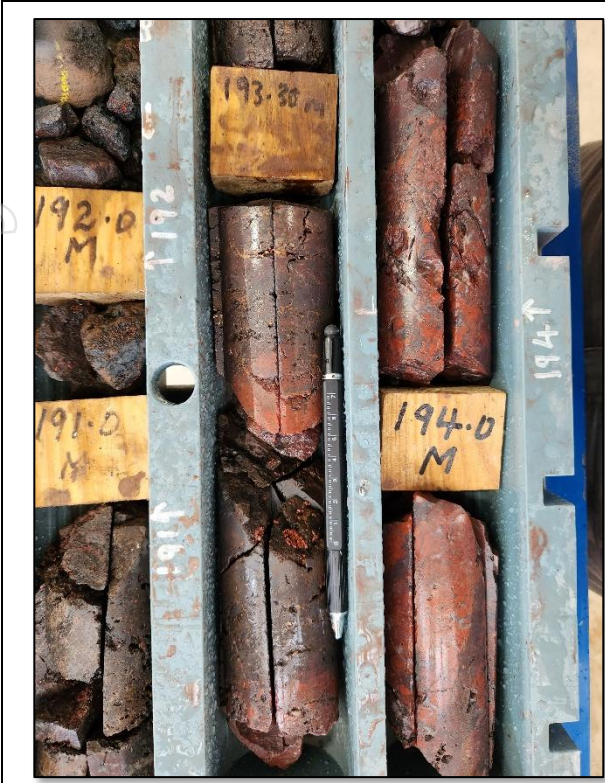
IMAGE 4 a and b: Hematite, quartz, jasper, copper sulphide, copper breccia (BBDD0050 @194m).
