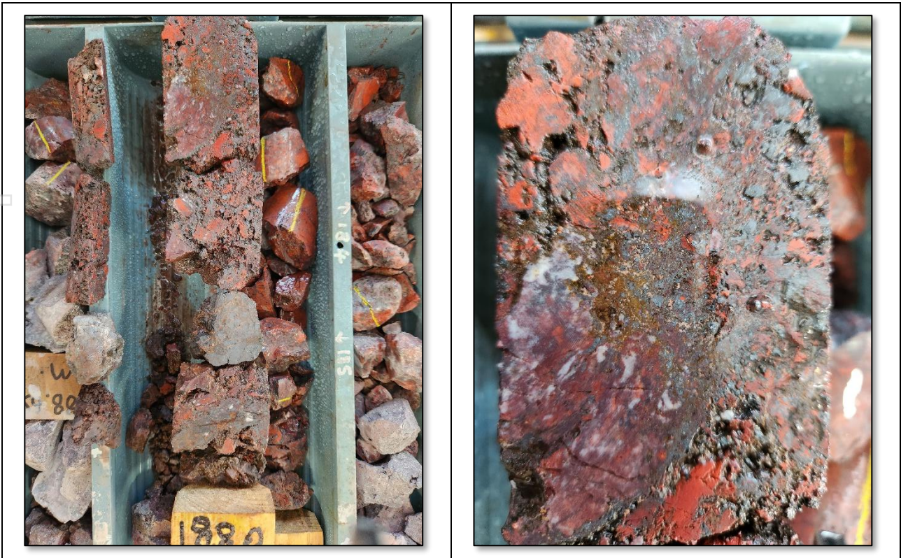
IMAGE 3 a and b: Hematite, quartz, jasper, copper sulphide, copper breccia (BBDD0050 @188m).
