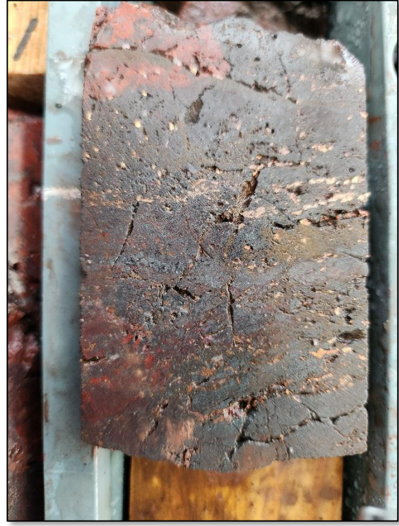
IMAGE 5 a and b: Hematite, quartz, jasper, copper sulphide, copper breccia (BBDD0050 @195m).
