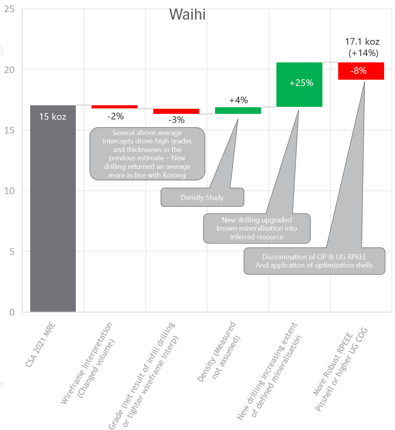
Figure 7. A waterfall chart showing changes from the previous Waihi MRE. New drilling did not match some of the higher grade intercepts that were driving sections of the 2021 estimate. New density data resulted in a small increase in tonnes, but there was very little new drilling beyond the extents of the old mineralisation model for Waihi. Much of the mineralisation modelled in the old estimate did not constitute a resource due to lack of drill density and therefore confidence. The largest increase in contained ounces is from infill drilling upgrading these zones into Inferred resource.
