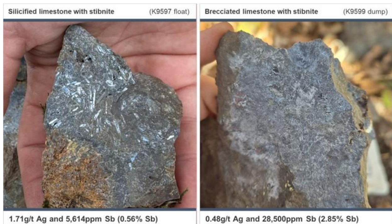
Figure 4: Red Rock Prospect – Dump and grab samples from historic workings, note visible radiating stibnite ( Sb_2S_3 ) crystals (refer Figure 2 for sample locations).
