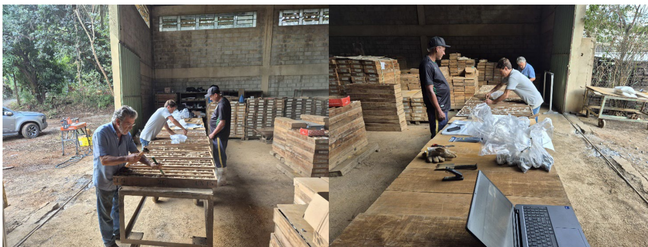
Photo 3 & 4: Consultant geologists and field technicians preparing Serra Negra diamond drilling core for sampling.
