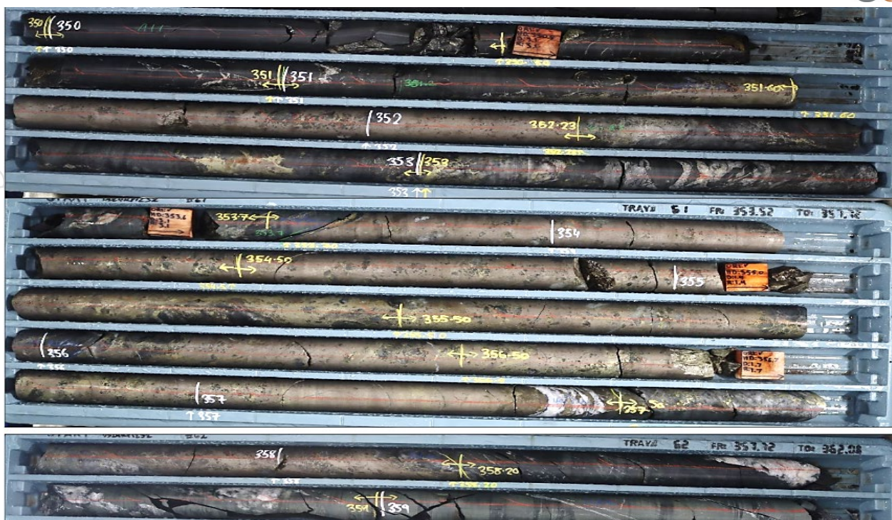
Figure 5- ~6.65m interval of massive and semi massive sulphides overprinting quartz veining from 351.2m, comprised of pyrrhotite (60%) and semi massive chalcopyrite (15%) and pyrite (5%). True width of the interval is estimated to be approximately 50% of the visually logged intercept length.
