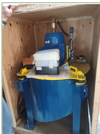
Figure 2 –Preparation of Falcon gravity concentrator for shipment
