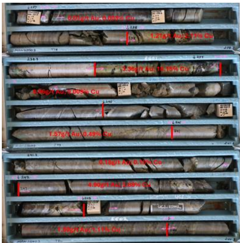
Figure 1: High grade primary copper-gold mineralisation from MRN25003 (From 238m) - 6.0 metres at 2.51% copper, 1.77 g/t gold
