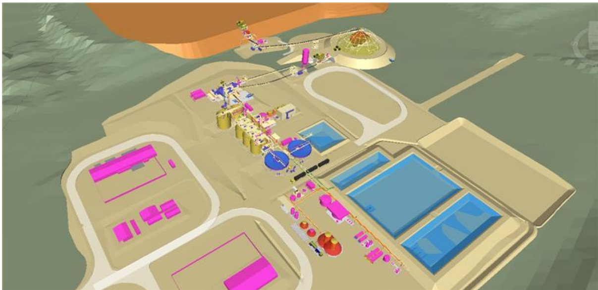
Figure 5: Indicative 3D model of the new 3.0 Mtpa mill
