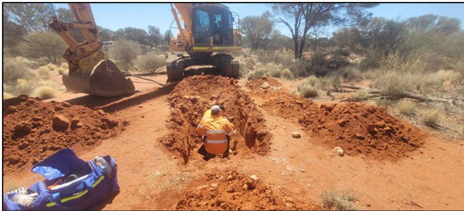
Figure 14 Sample collection for Geotechnical test work for Heap Leach Pad.
