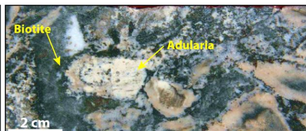
Breccia with K-feldspar (orthoclase or adularia) altered clasts with secondary biotite in-fill (ALN001, 333.3m).
