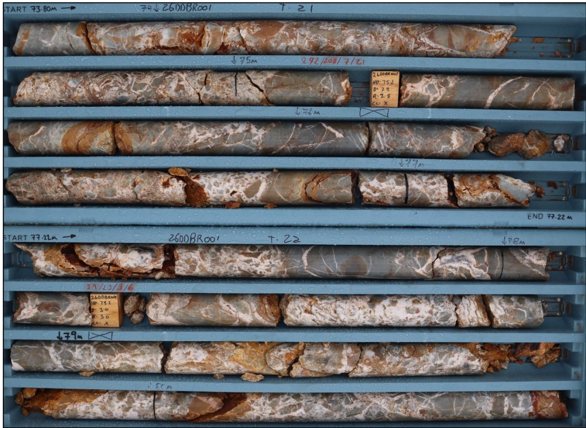
Figure 6: 26DDBR001 73.8 – 80.6m quartz cemented breccia (weathered/oxide zone).
