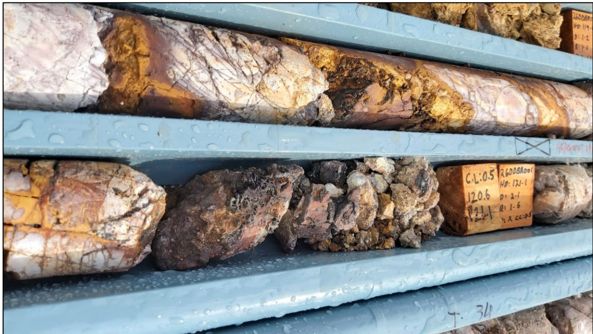
Figure 7: 26DDBR001 119.0 - 120.6m Gossanous iron-oxide boxworks textures due to oxidised sulfides.
