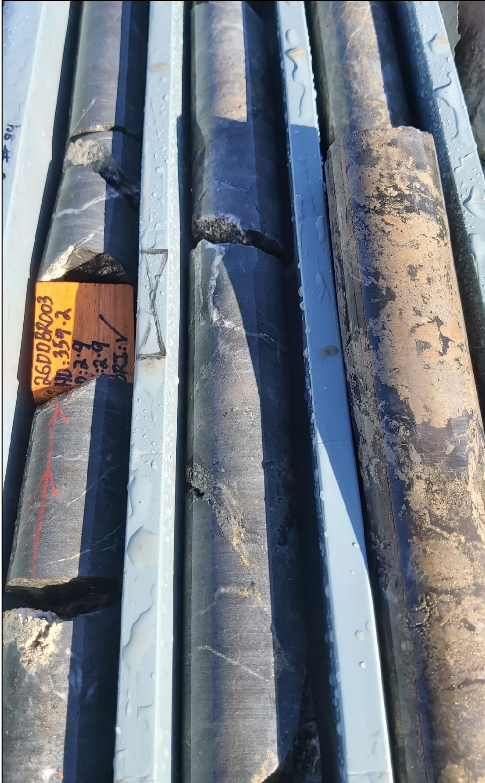
Figure 12: 26DDBR003 Morning sun on massive sphalerite in drill core (right), at 360.6m to 361.0m.
