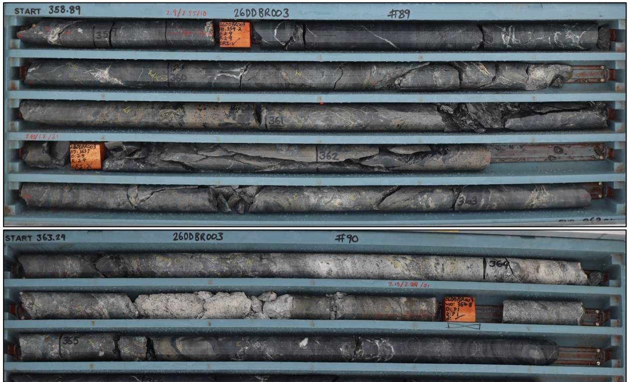
Figure 10: 26DDBR003 Massive & semi massive sulfides, sphalerite and pyrite.
