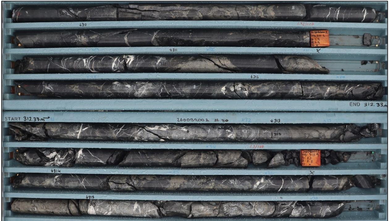
Figure 8: 26DDBR002 a section of the semi-massive and stringer sulfide zone, pyrite and sphalerite, 309-316m.
