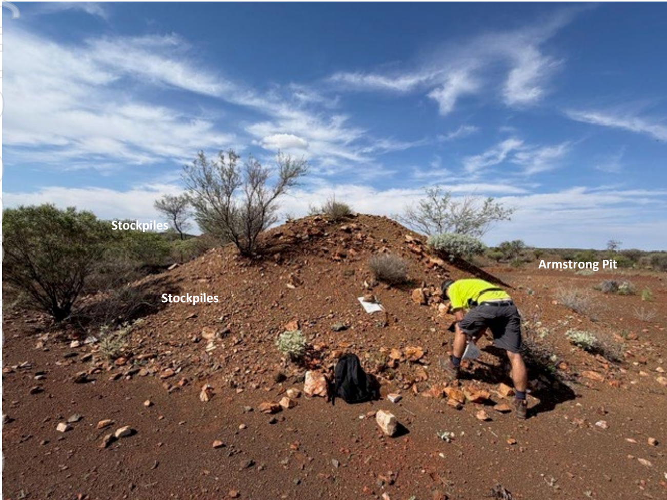
Photo 2: Resampling quartz veins at the Armstrong workings and stockpiles 6.07g/t & 3.21g/t Au.
