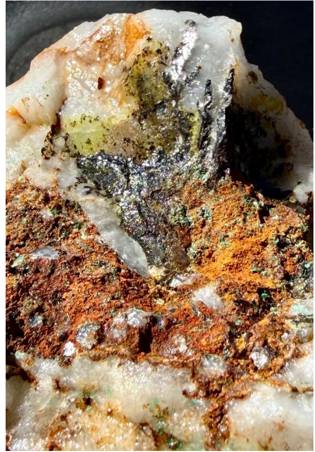
Photo 2. Coarse sprays of acicular wolframite in quartz with malachite and limonite gossan, FOV 5 cms.
