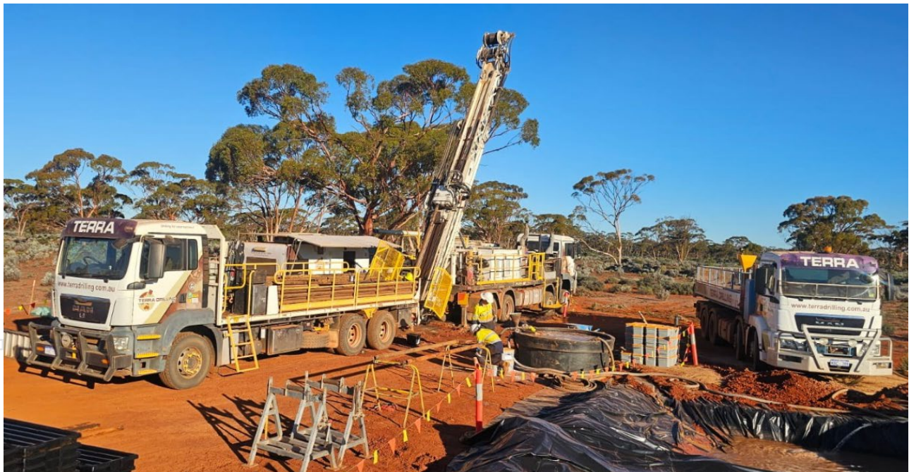
Figure 1. Diamond Drill Rig on Site at the EIS hole at the Kanowna Gold Project
