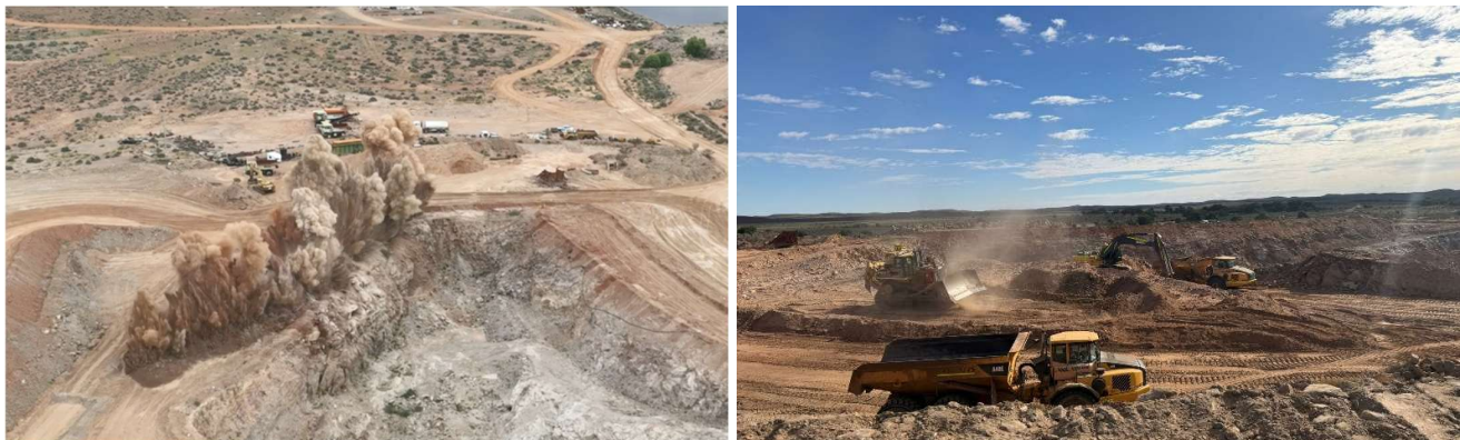
Figure 2 – Drill/blast and truck/shovel operations underway at the Pinnacles Mine
