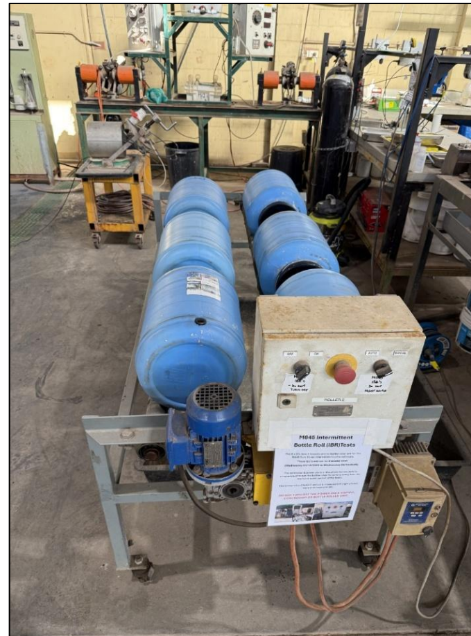
IBR Metallurgical Testing two sample composites across three grind sizes (6.3mm, 3.35mm and 2mm)
