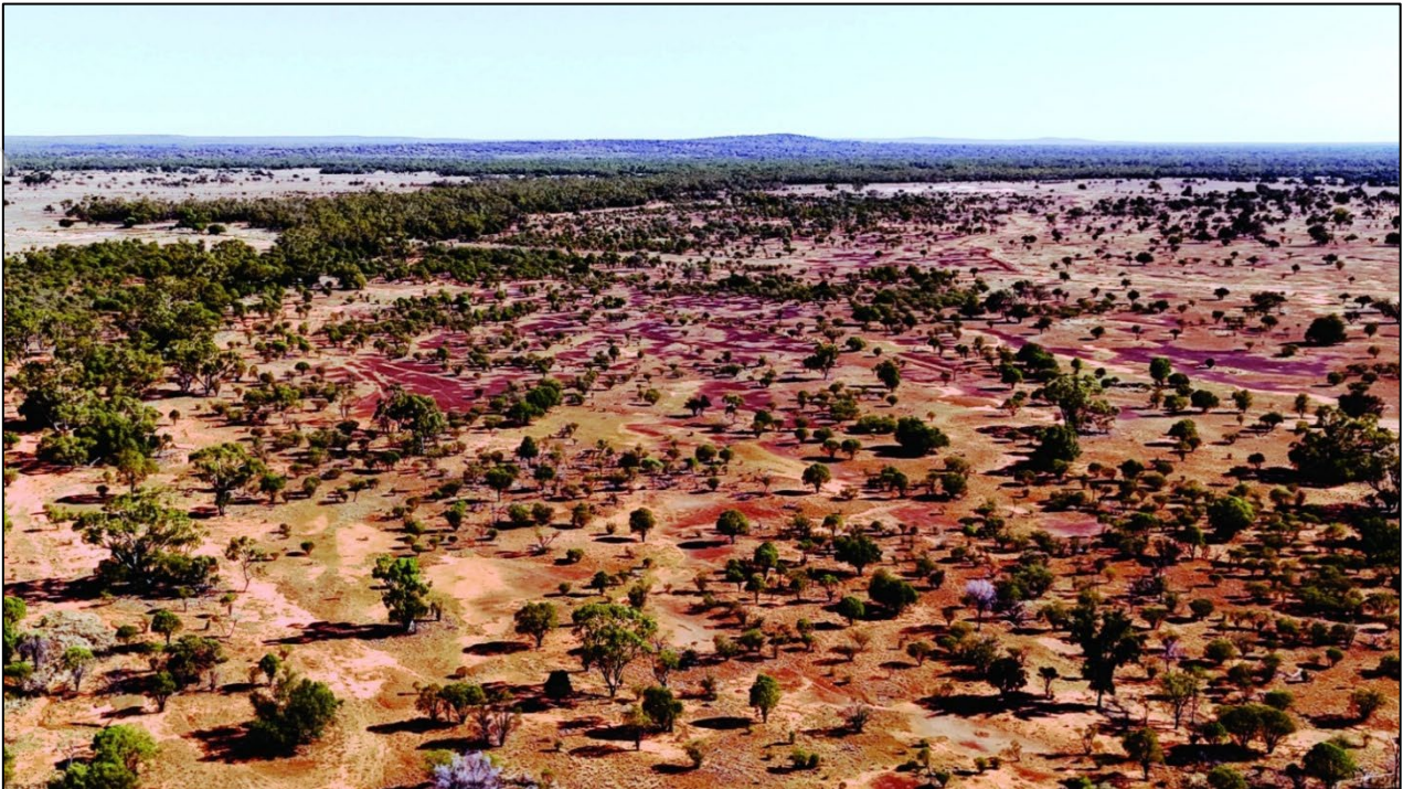
Figure 3: Blind Freddie prospect area showing widespread ferruginous lag derived from outcrop and sub-outcrop, anomalous in copper. Low hill on RHS is Mulga Downs sandstone cover
