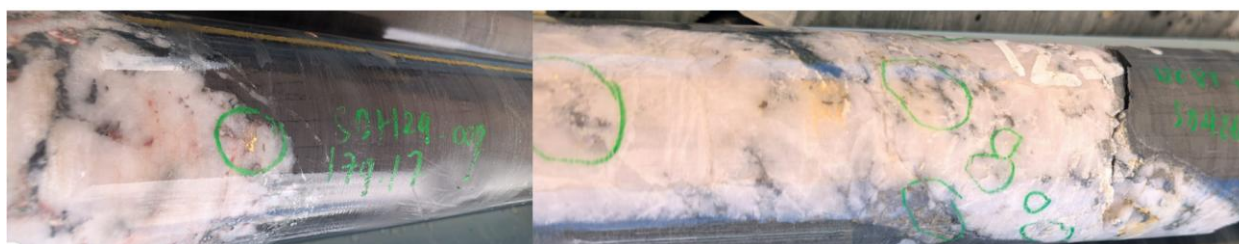
Plates 1 and 2- Visible gold intersected in SDH26-009, up dip from the previous Link Zone intercepts
