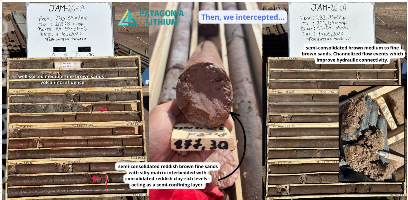
Figure 1. JAM 26-07 core sample 270m to 293m gravels and sand contributing to high porosity, the clay aquitard will stop lower conductivity brines impacting the lithium high conductivity brines
