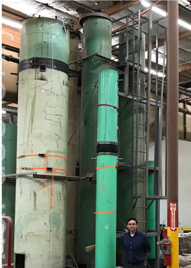
Column testing of ore at KCA, Reno
