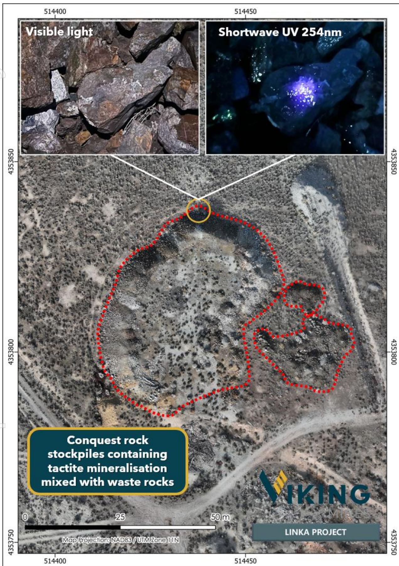
Figure 2; Map showing the Conquest rock stockpile and photographs of scheelite response under UV light. Estimated abundance is between 0.4-1.0% WO_3 . Laboratory analysis required to confirm grade of % WO_3 with results expected in Q3 2026.
