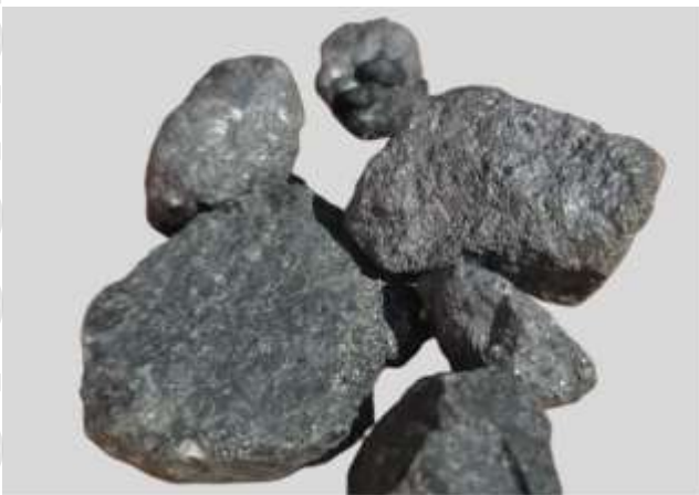
Figure 2 – Galena and sphalerite mineralisation percussion chips intersected in BTPRC010 (90 – 91m)
