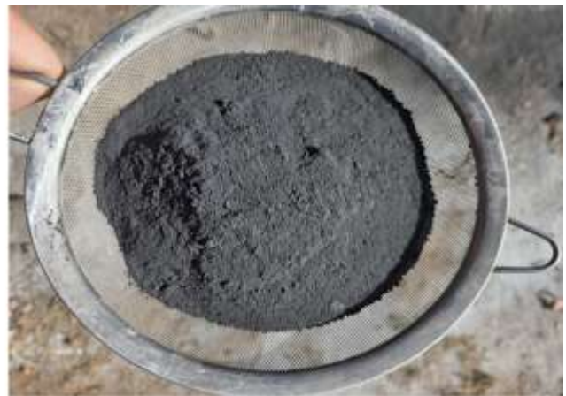
Figure 2 – Galena and sphalerite mineralisation percussion chips intersected in BTPRC010 (90 – 91m)
