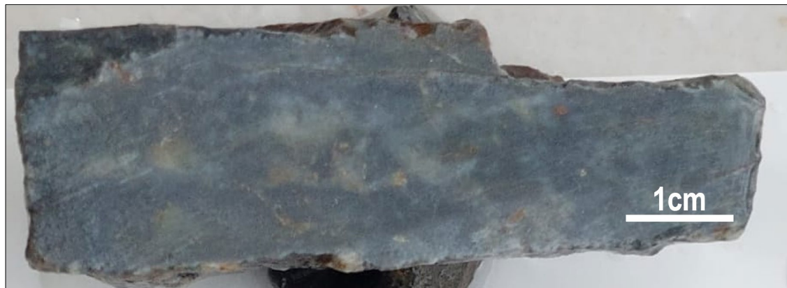
Photo 4. 7.12g/t Au & 0.39% Sb rock sample from Doyle's Prospect (ER0174) with quartz-carbonate-sulphide vein and abundant arsenopyrite-?sulphosalts within granite from mullock pile around historical workings.
