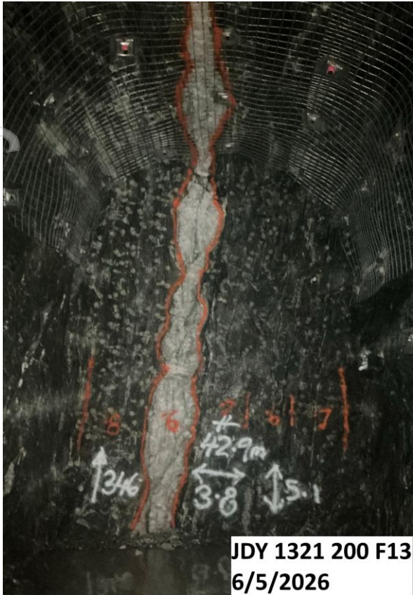
Figure 1: Face photo from Judy North 1321 level (average face grade: 4.0m @ 25.3g/t Au, inc. 0.6m @ 145.6g/t Au).
