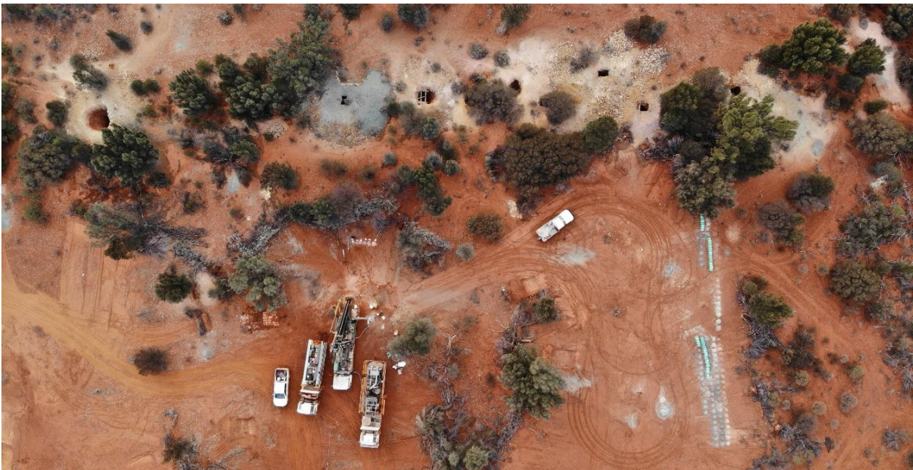
Figure 2: Drone image of drilling at Metzke's Find in 2020 showing part of the line of historical workings.
