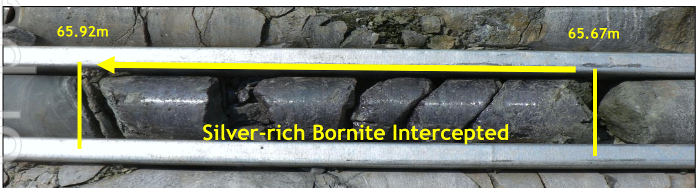
Above: Bornite in diamond hole ACRD029 returned 1.13m @ 21.58% Cu, 1,023g/t Ag from 65.39m including 0.25m @ 60.98% Cu, 2,833g/t Ag from 65.67m (ASX release 5 November 2010)
