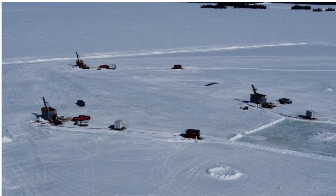
Figure 2: Three drill rigs completing Golden Eye resource conversion program on the engineered ice pad (March 2026).
