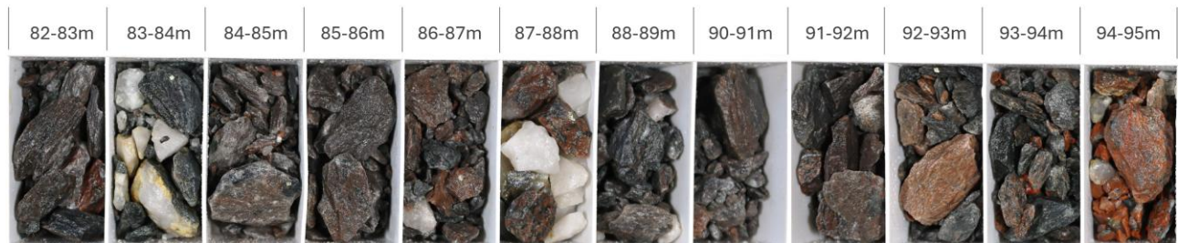
FIGURE 2: NMWBRC26-825 – 12M AT 3.81G/T AU INCLUDING 1M AT 26.53G/T AU FROM 82M (WITHIN A BROADER INTERCEPT OF 19M AT 2.51G/T AU FROM 76M)
