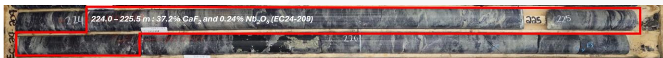
Figure 4. Example fluorspar (dark purple) mineralization in host dolomite carbonatite (light grey) at the Flux Fluorite Zone, Mallard Prospect (EC24-209; 2024 drilling campaign). The interval shown contains approximately 37% fluorspar (fluorite), with the remainder being predominantly dolomite.
