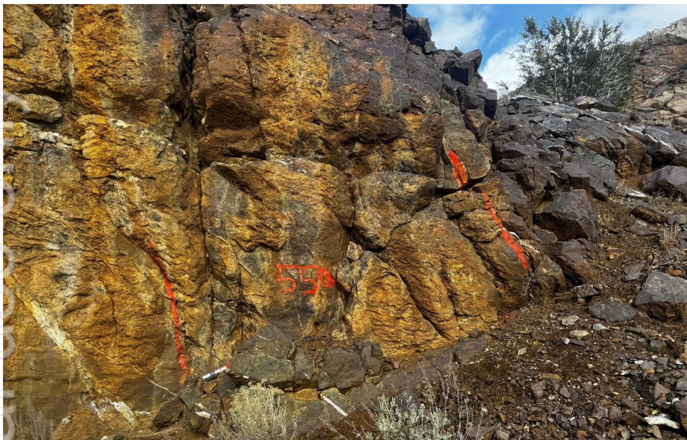
Figure 3 – Channel sample ID 1080550 of limestone skarn that returned 4,191 ppm W from the northern section of the historic Garnet Mine, Alder Mining District, Elko County, Nevada. Five (5) holes are designed to test the immediate area.
