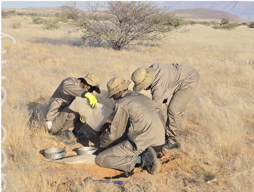
Image 2: Sampling team in the field at EPL 7626 weighing sieved soil samples in preparation for bagging the samples for analysis with XRF, LIB's and Pellet Press.
