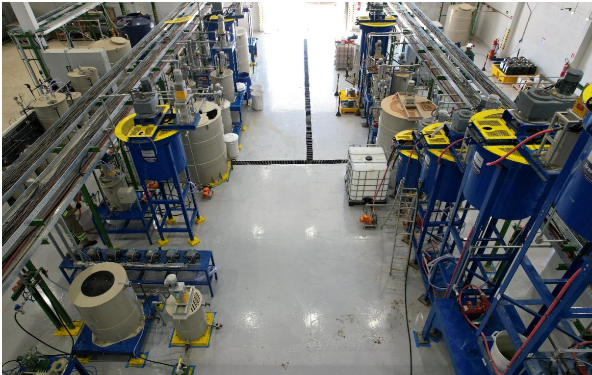
Figure 6: The Demonstration Plant replicates the Colossus project flowsheet. (Top right) Desorption stage, (bottom right) Counter Current Decantation ('CCD') stage to maximise rare earth elements ('REE') recovery and ensure spent clay meets all environmental limits for mining pit rehabilitation, (top left) Impurity removal stage, and (bottom left) MREC precipitation and filtering stage.
