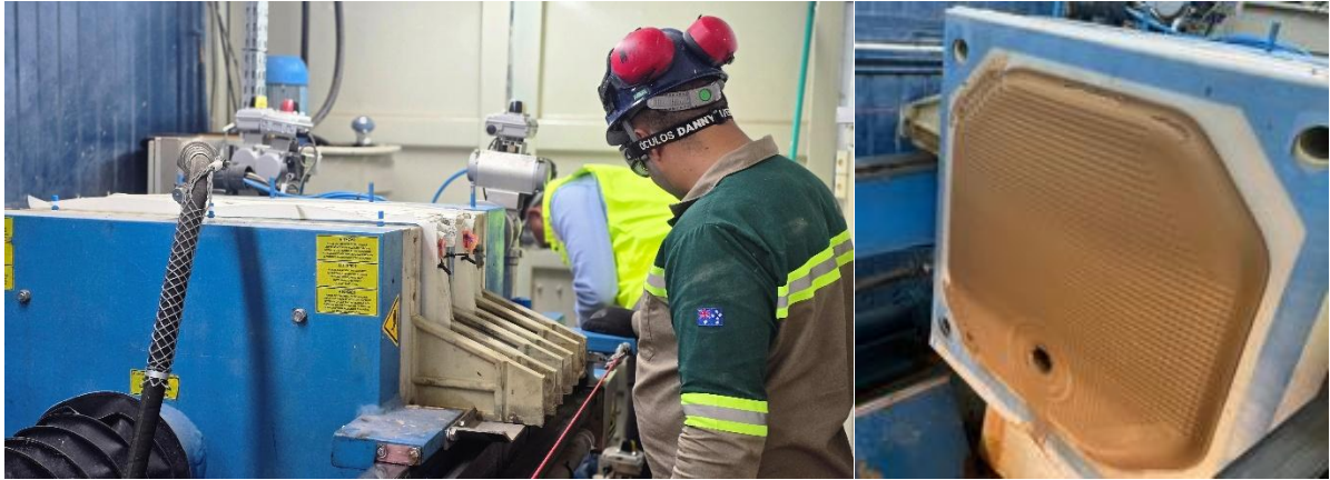
Figure 8: All major packages have been sourced from suppliers that are tendering the LLI packages for the Colossus Project. Pictured: (left) Residue pressure filter, (right) formed up filter cake during operations where various moisture content, membrane pressures etc. are being evaluated.
