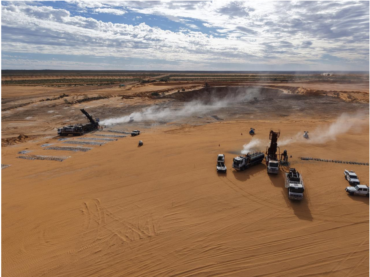
Figure 1: Two RC Drill Rigs from Raglan Drilling on-site at Iguana as of 10 January 2026. Imagery looking south, with the Jamaican Rock test pit in background
