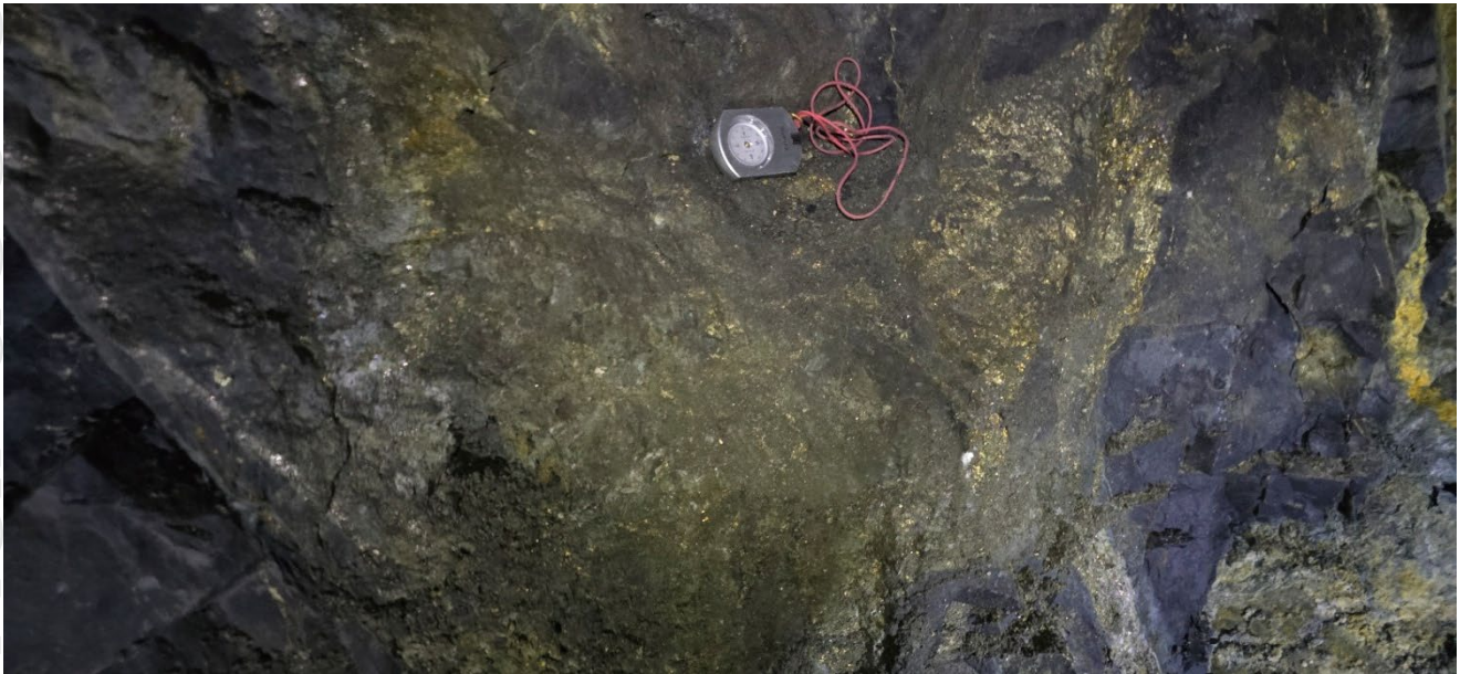
Photo 1. Underground mineralisation from the La Martuca Prospect, showing massive, vein, and matrix copper sulphide hosted in structurally controlled quartz-sulphide veining and breccia (sample 26LMR00030, returned 5.32% Cu - see Tables 1 and 2 and Appendix 1).
