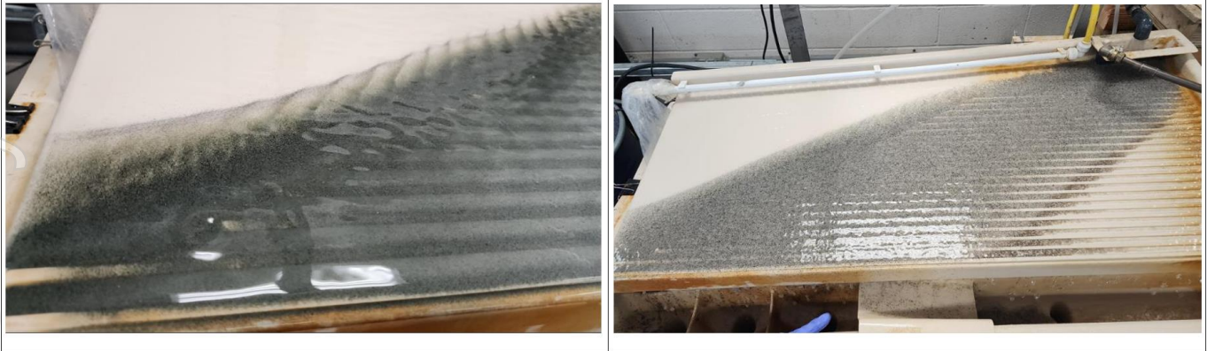
Figure 4: Testwork images on Tantalum recovery across industry standard Wilfley tables
