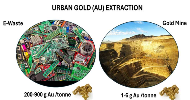
Figure 2 – Gold Content in E-Waste Compared with Gold Mines
