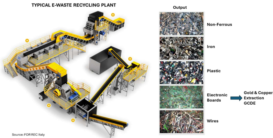
Figure 3 – Typical E-Waste recycling plants separating electronic boards
