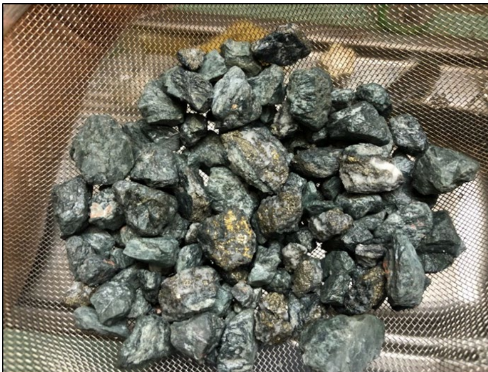
Figure 9: Burringa discovery drill hole, aircore rock chips from JAC0089 at 60m, grading 2m at 0.5% Cu and 0.12g/t Au from 60m to EOH, with quartz-chlorite-sericite-pyrite alteration and visible chalcopyrite mineralisation in diorite, photo Glen Diemar January 2019.
