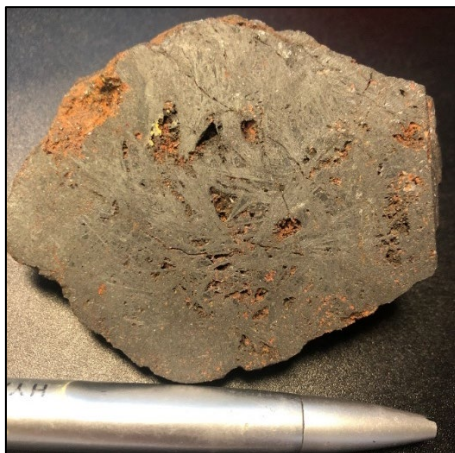
Figure 11: Burringa East rock float sample of bladed magnetite 2.5g/t Au, 0.4% Cu, 112ppm Mo, 26ppm Bi, 3ppm Te (17R1043).
