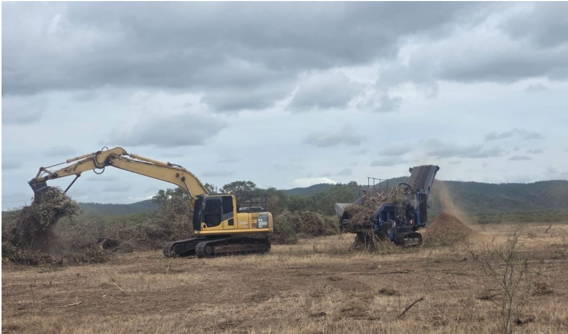
Mechanical Harvesting and Chipping of Feedstock prior to Pyrolysis testing by Pyrocal
