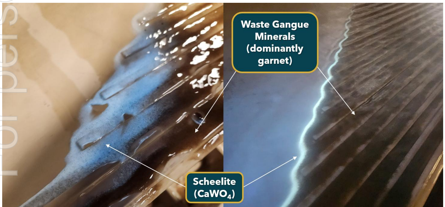
Figure 1; Photo showing separation of scheelite (white) from waste minerals (dark brown) during Wilfley table gravity concentration stage. Wilfley concentrate feeds into the Mozley table cleaning stage. Assayed grade of Mozley table concentrate is 66.6% WO 3 .
