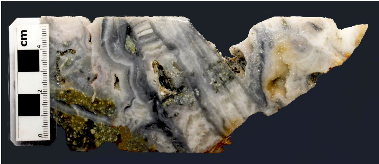
Figure 2. Diamond drill core, TSD-26-018, 224.4m at Gufinis. Multiphase epithermal colloform-banded vuggy quartz vein breccia; part of an interval, 1m at 14.32 g/t Au (Table 1).
