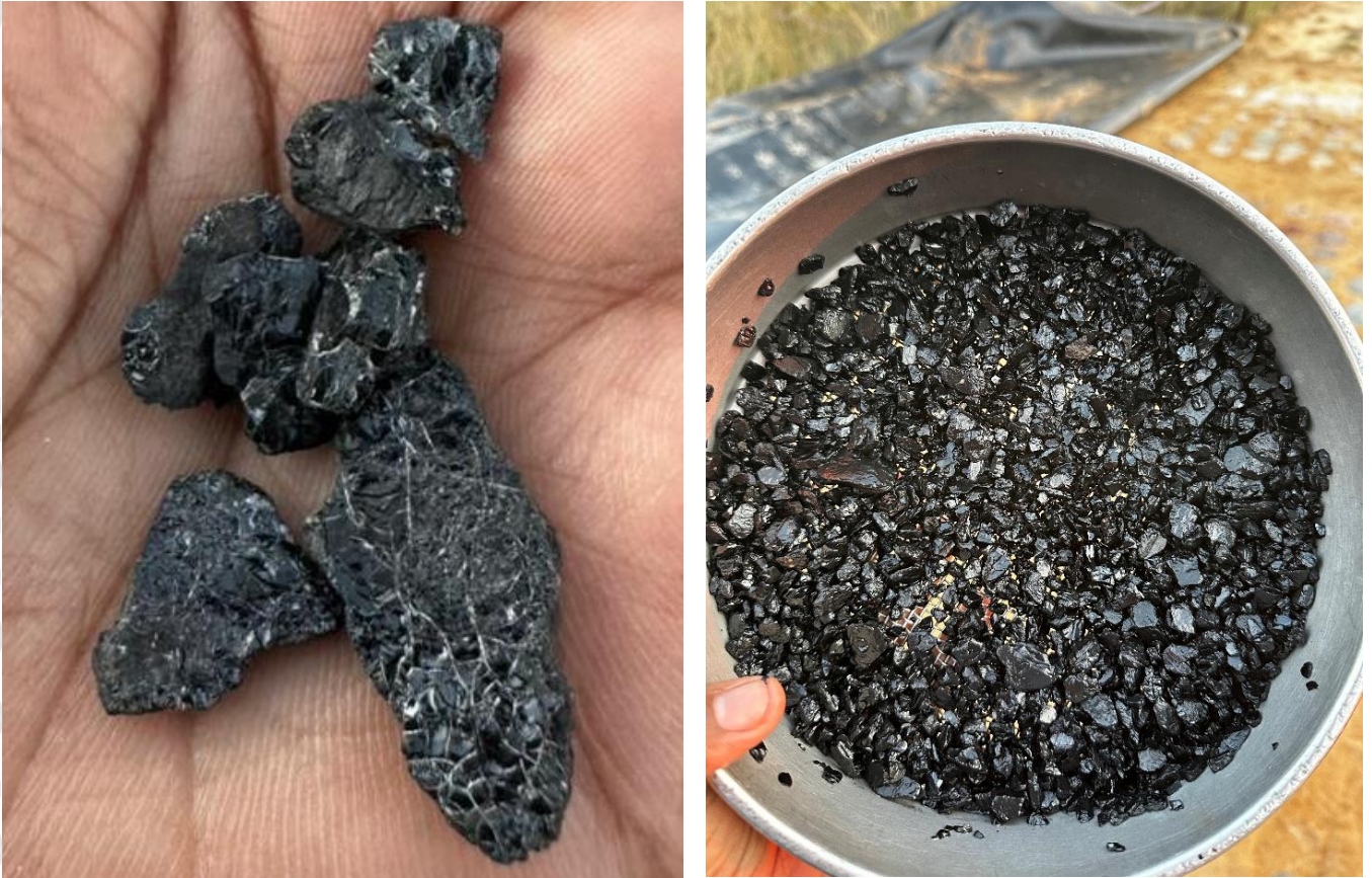
Figure 1. Serowe seam coal rock chips – bright coal with well-formed cleats (Source: Botala)
