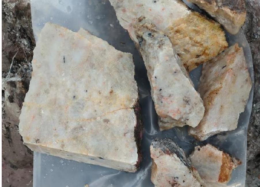
Figure 3: Channel sample at the newly discovered Cosma Caesium Pegmatite, assaying 0.5 m at 16.43% \text{Cs}_2\text{O} .
